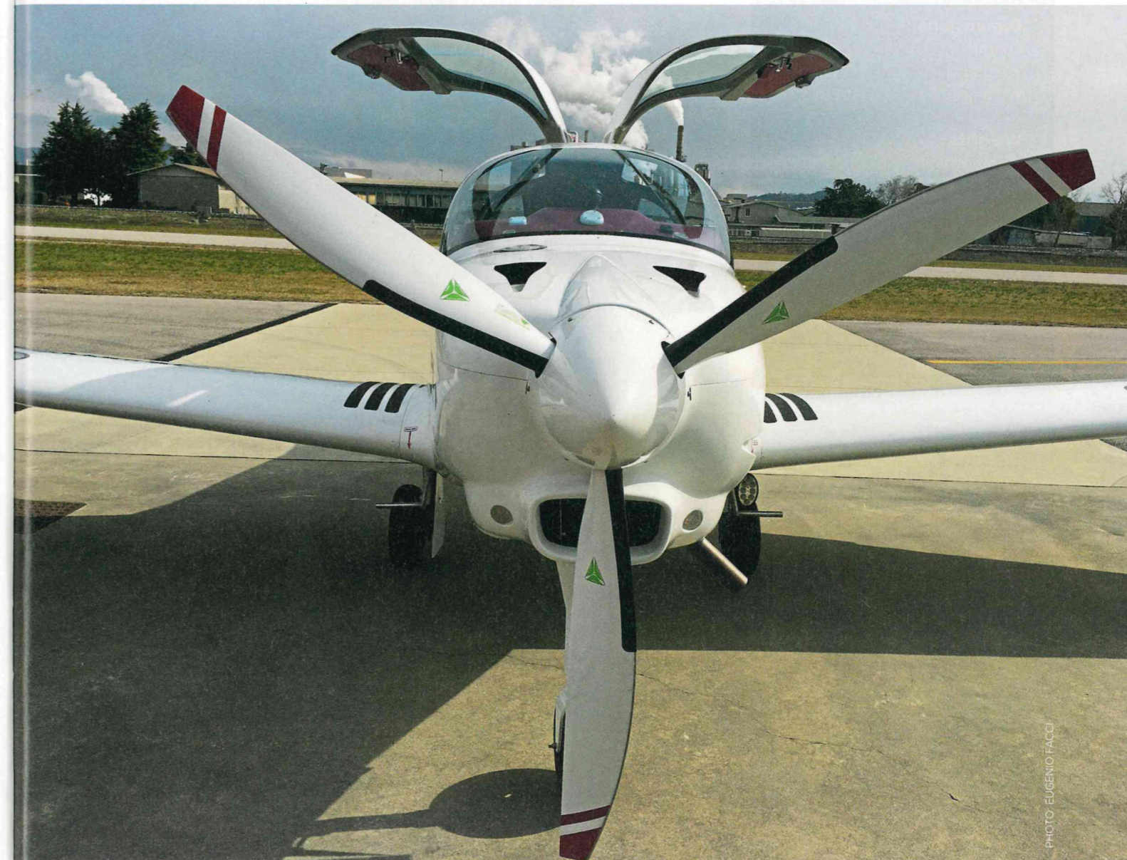
▲ You enter the aircraft from the front of the wing, aided by a small metallic step. The gull-wing doors make entry easy
