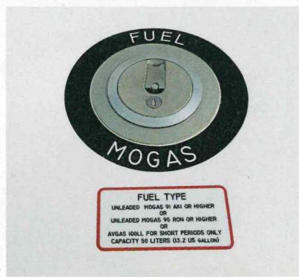
▲ The Pioneer 400-915 iS runs on mogas, but it can use leaded avgas for short periods of time if needed
