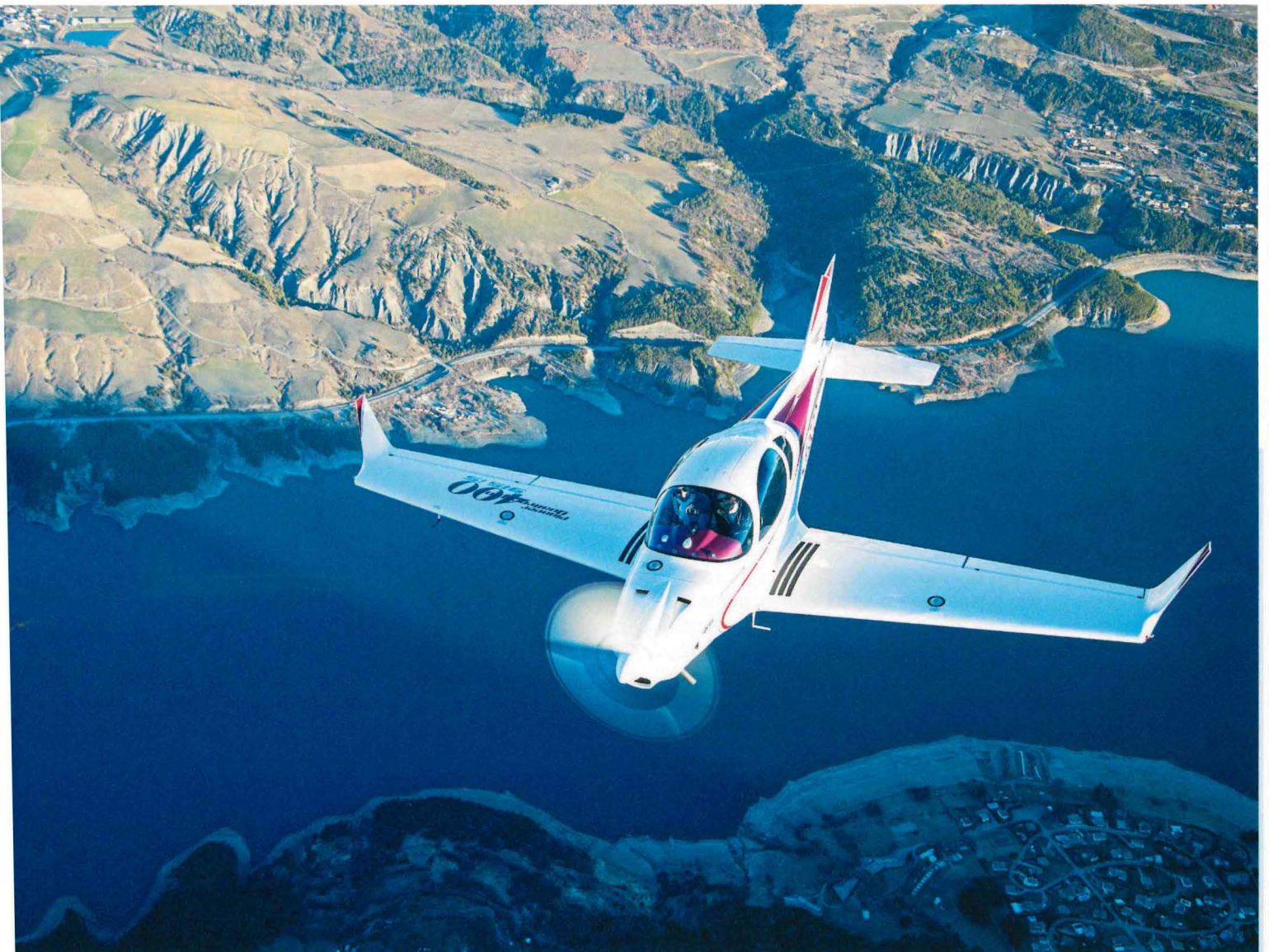
▲ Sleek aerodynamics give the 400 a high cruise speed, while the fairly large wing area allows the aircraft to operate from short strips
