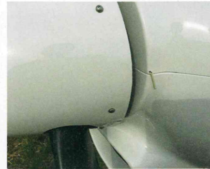
▲ The cowling can be opened quickly by one person by removing two pins
