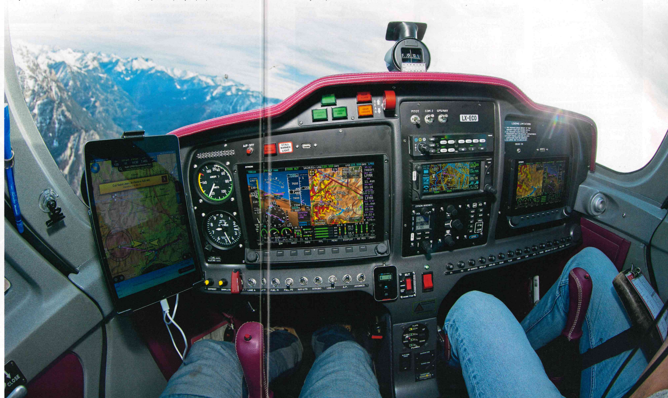
▲ The autopilot has a variety of modes (NAV and V-NAV for instance) that allow you to do airline-style navigation
