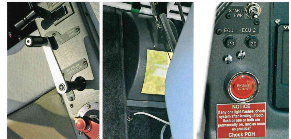
CLOCKWISE FROM TOP LEFT: undercarriage lights, closely spaced and identically-shaped throttle and propeller plungers, and (almost hidden below) flap switch/indicator; centre console brake T-handle, elevator and rudder trims, and parking brake valve; and the quality Andair tank selector; independent ECU CBs and indicator lights, with starter switch below; the little window that allows visual confirmation that the nosewheel is retracted; and the emergency manual undercarriage extension crank in position
